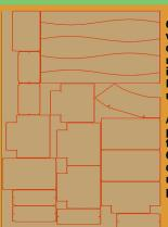
QuickDuct CAM Master's Advanced Shape Nesting automatically nests parts side by side and rotates them to match interlocking angles and contours.
