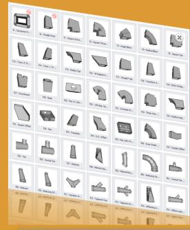
If you frequently cut similar parts with varying dimensions, Shop Data's Macro Programming Utilities allows you to build your own dimensionable shape library! Now you don't have to redraw every variation of a given part type. This feature works great for multiple component assemblies such as containers, enclosures, curbs, even your own HVAC fitting design!
